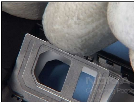
32. Turn the assembly and open the SIM lid.
