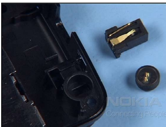
24. Remove the MICROPHONE and the DC JACK.
