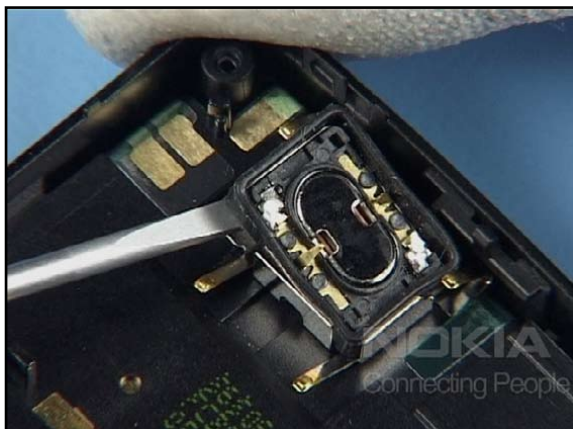
25. Carefully lever out the EARPIECE ASSEMBLY.
