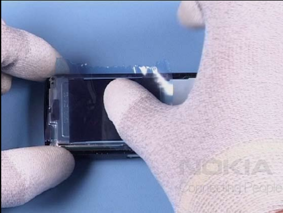
13. Cover the display with a film.
