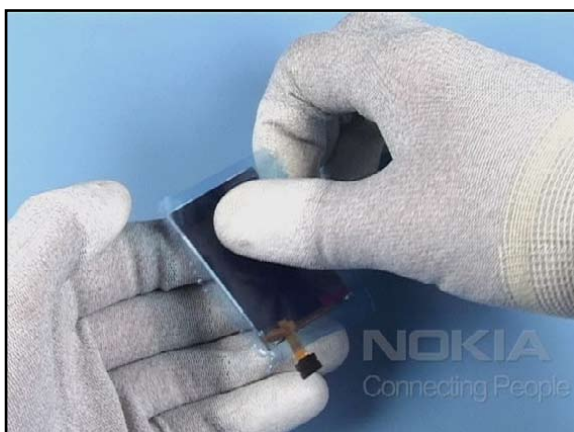
23. Cover the display with a film again.
