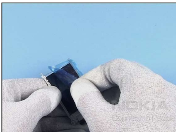
21. Peel up the protective film.
