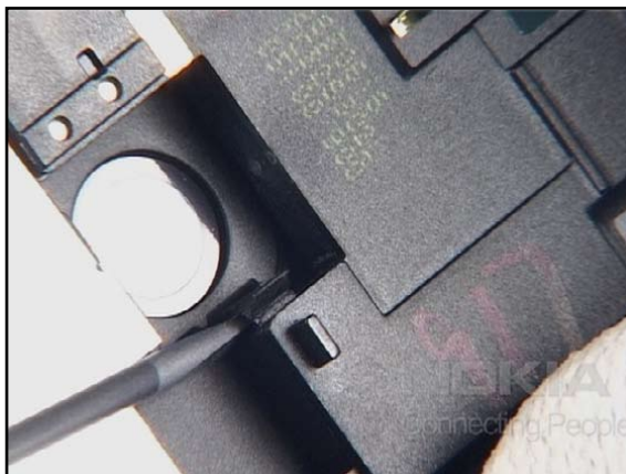
26. Carefully unlock the clip securing the PLASTIC CHAMBER.
