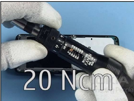
15. Set the correct torque.
