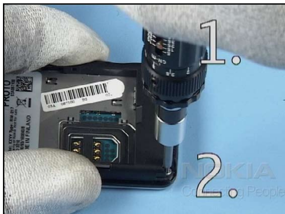
18. Tighten both screws of the C-COVER in the order shown, too.
