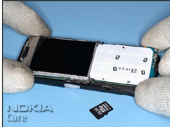
14. Place the assembly onto the B-COVER.
