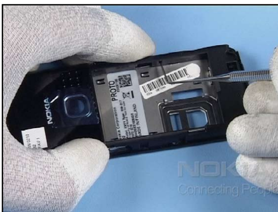
34. Use the dental tool to push out the last clips.
